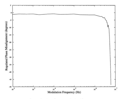
Figure A.6. Phase alignment vs. baseband frequency
