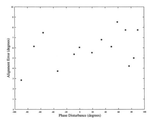
Figure 5.25. Phase alignment performance for a 500mV amplitude, 10 kHz square wave.
