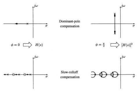
Figure 4.4. Root locus plots for dominant-pole and slow-rolloff  $\left(\frac{k}{\sqrt{s}}\right)$  compensation.
