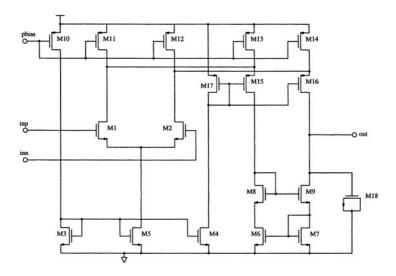
Figure 5.15. Opamp\_nL, a single-ended op-amp for high common-mode inputs.
