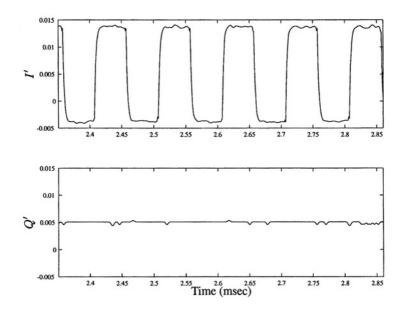
Figure 5.44. Step response of aligned, uncompensated system.
