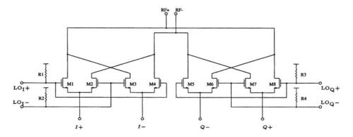
Figure 5.31. Upconversion mixer. All transistors are sized  $2 \times 50.4/0.24$ , all resistors are  $10k\Omega$ .
