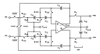
Figure 5.16. Switched-capacitor, non-inverting integrator for phase alignment system. Switches are complementary: NMOS 2/0.24, PMOS 6/0.24.
