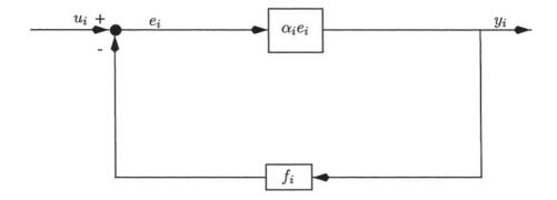
Figure 2.2. Linearized static model of amplifier stage.
