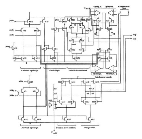
Figure 5.29. Loop driver amplifier.
