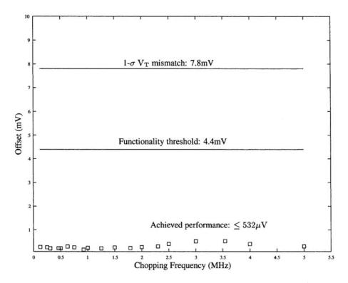
Figure 5.26. Effective output offset,  $\delta_0$ , of the chopper-stabilized multipliers of figure 5.12.
