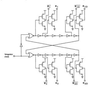
Figure 5.19. Circuit for generating clock phases.
