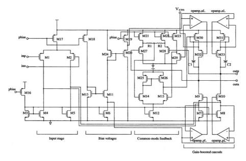
Figure 5.13. Op-amp\_d1, a fully differential op-amp for the S.C. integrator.
