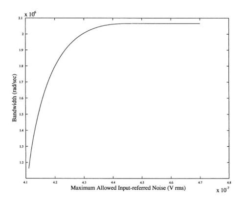
Figure 2.6. Maximum bandwidth versus limit on input-referred noise.
