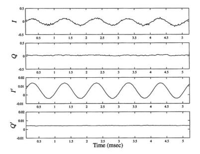
*Figure 5.39.* Comparison between predistortion inputs and downconverter outputs for no misalignment.
