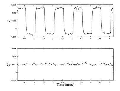
Figure 5.45. Step response of aligned, slow-rolloff compensated system.
