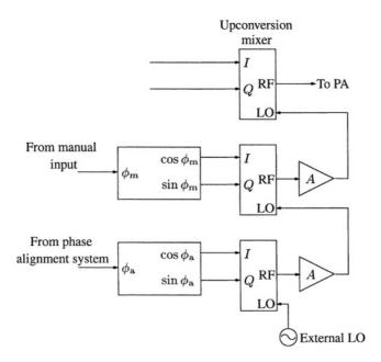
Figure 5.4. Phase alignment by phase shifting the local oscillator.
