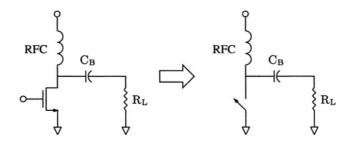
Figure 3.1. A high-efficiency power amplifier.
