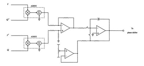
Figure A.3. Phase error computation and integration.
