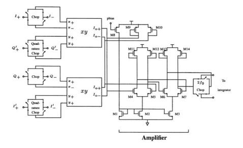
Figure 5.12. Phase error computation.
