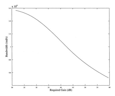
*Figure 2.8.* Maximum bandwidth versus required closed-loop gain. Maximum input-referred noise = 4.15e-7 V rms.
