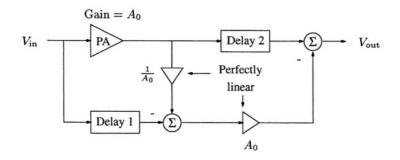
Figure 3.4. Feedforward linearization.
