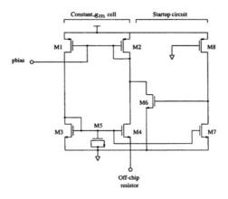
Figure 5.37. Constant\_gm cell, which establishes the voltage 'pbias' for the entire chip.
