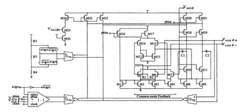
Figure 5.20. Constant 1-norm controller: circuit realization of figure 5.7.
