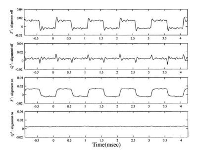
Figure 5.28. Illustration of phase alignment stabilizing the closed-loop CFB system.
