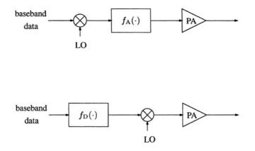
Figure 3.2. Using predistortion to linearize a power amplifier.
