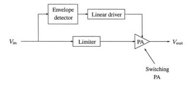
Figure 3.5. Envelope elimination and restoration.
