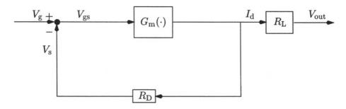
Figure 2.14. Modification for nonlinear static model.
