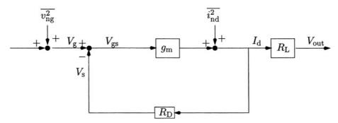
Figure 2.17. MOSFET gate and drain noise.
