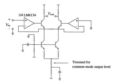
Figure B.1. Converting from single-ended to differential signals.
