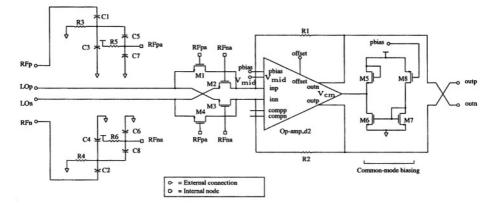
*Figure 5.33.* Potentiometric downconversion mixer, together with biasing and capacitive RF attenuator.
