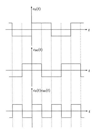
Figure 4.9. Graphically computing  $c_0(t)c_{90}(t)$ .
