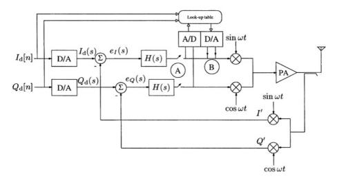
Figure 5.2. Cartesian feedback used to train a predistorter.
