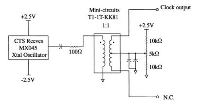
Figure B.2. The on-board clock reference.
