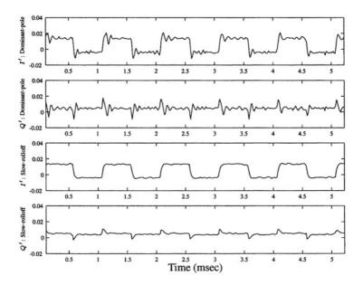
*Figure 5.46.* Step response comparison between dominant-pole and slow-rolloff compensated systems for 90-degree misalignment.
