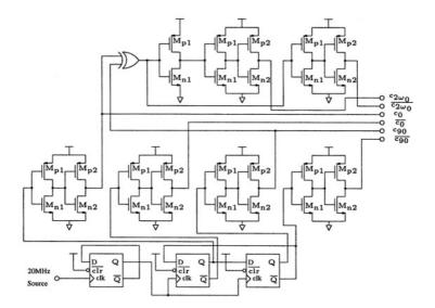
Figure 5.17. Chopping clocks derived from off-chip source.
