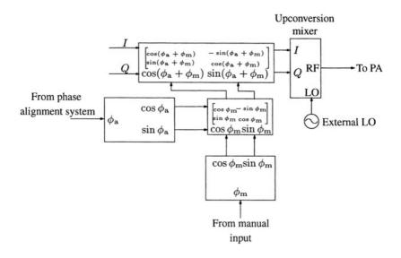
Figure 5.5. Phase alignment by rotating the baseband symbol.
