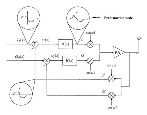
*Figure 5.1.* The predistorting action of Cartesian feedback.
