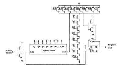
Figure 5.18. Integrator clock, which transitions on the trailing edge of the external 20MHz source.
