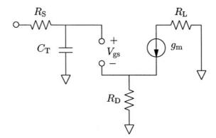
Figure 2.15. Modeling dynamics using the Miller approximation.
