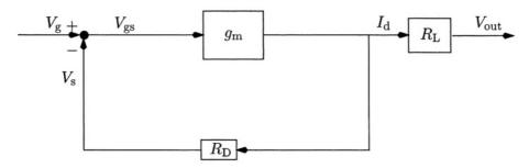
Figure 2.13. Source degeneration as a form of feedback.
