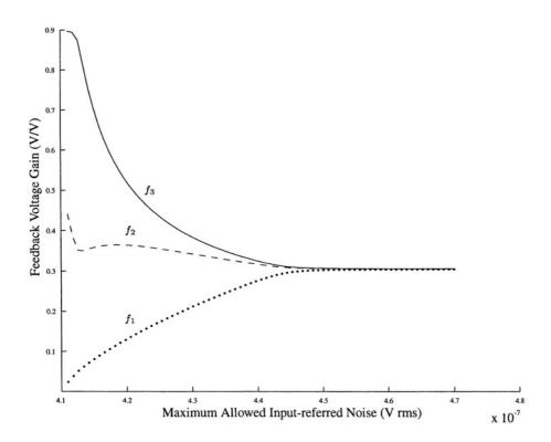
*Figure 2.7.* Optimal feedback allocation pattern, for maximum bandwidth with limit on inputreferred noise. Gain = 23.5dB.
