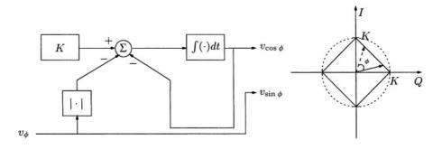
Figure 5.7. Analog rotation using the 1-norm.
