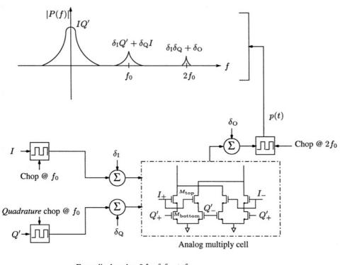
Error displaced to  $2f_0$ :  $\delta_I \delta_Q + \delta_O$ Error displaced to  $f_0$ :  $\delta_I Q' + \delta_Q I$ Product centered @ DC: IQ'
