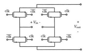
Figure 5.11. Commutating mixer for chopping. NMOS devices are sized 3/0.24, PMOS 9/0.24
