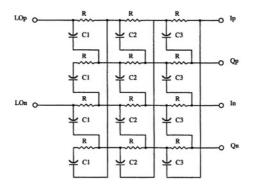
Figure 5.36. A three-stage polyphase filter.
