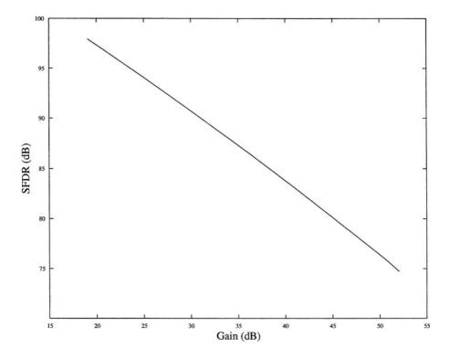
Figure 2.10. Maximum spurious-free dynamic range versus required gain.
