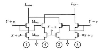
Figure 5.9. Basic topology for multiplier cell. All transistors connected to a y input are sized  $M_{top}$ , and all transistors connected to a x input are sized  $M_{bot}$ .
