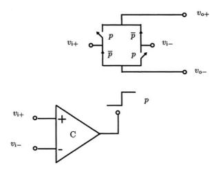
*Figure 5.8.* Using CMOS voltage switches and a comparator to realize a folding amplifier. Switches are closed when their respective control signal is high.
