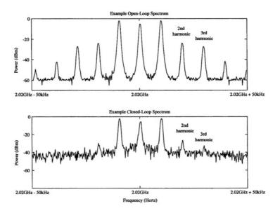
Figure 5.41. Frequency-domain example of linearization behavior.
