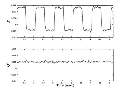
Figure 5.43. Step response of aligned, dominant-pole compensated system.
