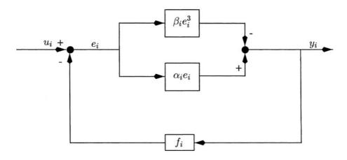
Figure 2.3. Nonlinear static model of amplifier stage.
