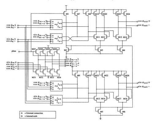
Figure 5.23. Computation of the rotation operator.
