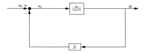
Figure 2.4. Linear dynamic model of amplifier stage.
