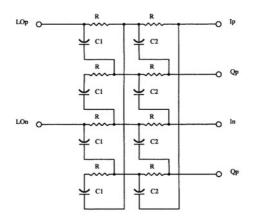
Figure 5.35. A two-stage polyphase filter.
