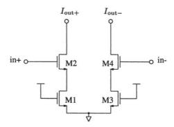
Figure 5.21. Differential transconductor.
