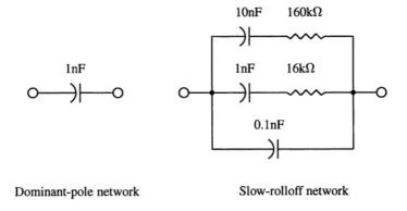
Figure 5.42. Compensation networks used in stability experiments.
