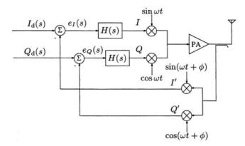
Figure 4.1. Typical Cartesian feedback system.
