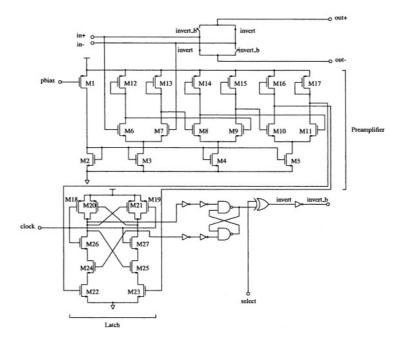
Figure 5.22. Folding amplifier for constant 1-norm controller.
