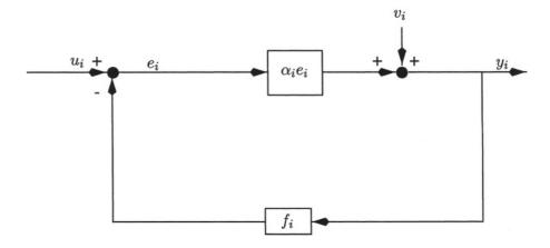
Figure 2.5. Static noise model of amplifier stage.
