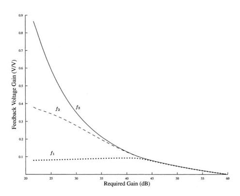
*Figure 2.9.* Optimal feedback allocation pattern for maximum bandwidth versus required closed-loop gain. Maximum input-referred noise = 4.15e-7 V rms.
