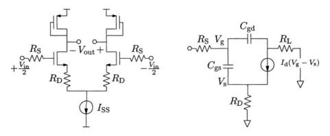
Figure 2.12. CMOS source-coupled pair and differential half-circuit.
